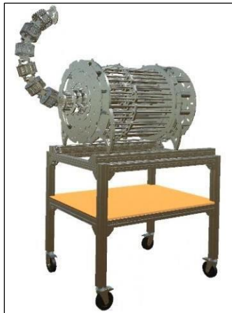
Figure 2. Tendon-Driven, Discrete and Hyper-Redundant Manipulator
