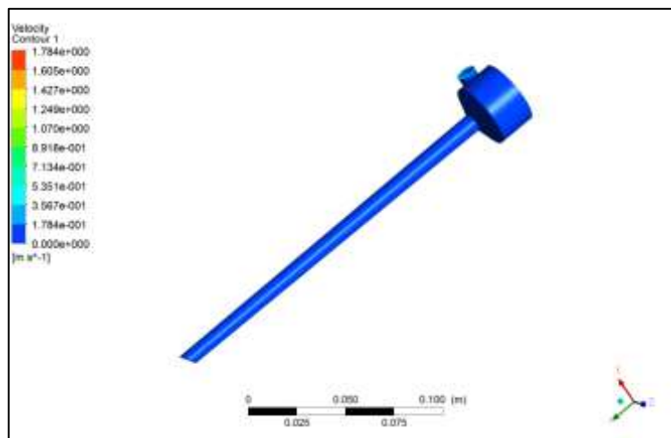
Figure 5. The best average velocity of spiral straight tip cannula, ST-Type 11
