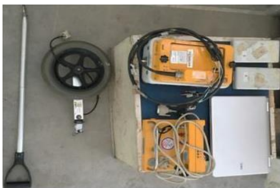
Figure 2. 800MHz MALA Ramac GPR
