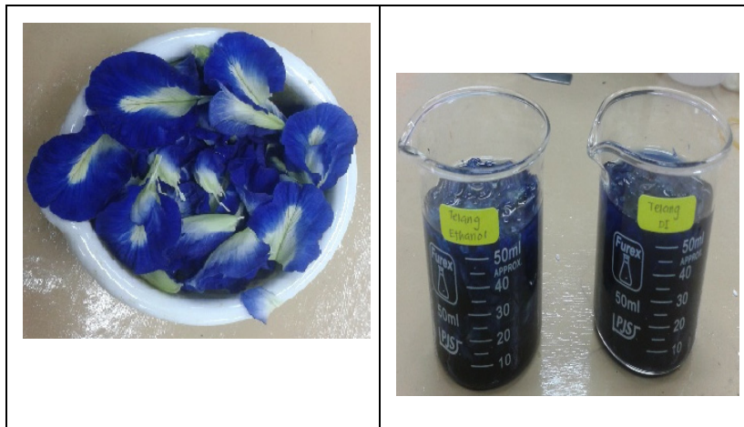
Figure 2: Preparation of blue pea dye sensitizer extract
