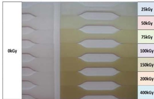
Figure 13: Visual effect of increased irradiation dose on PP samples
