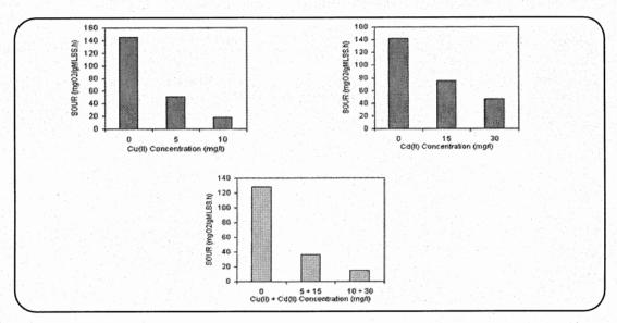
Figure 1. Inhibitory effect of heavy metals on SOUR in activated sludge microbes
