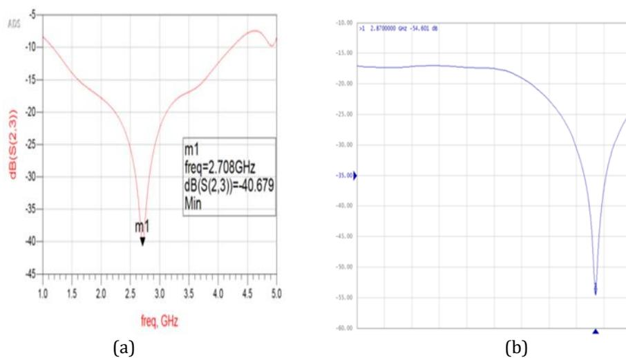
**Figure 9.** (a) Simulated result of isolation ( $S_{23}$ ) of four-way power divider (b) Measured result of isolation ( $S_{23}$ ) of four-way power divider
