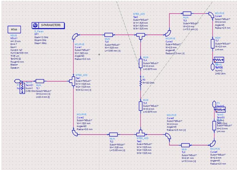
Figure 1. Two-way Microstrip Power Divider Design in Schematic Diagram.
