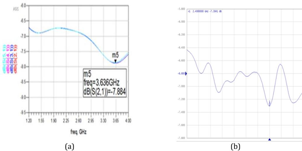
**Figure 8.** (a) Simulated result of insertion loss ( $S_{21}, S_{31}, S_{41}, S_{51}$ ) of four-way power divider (b) Measured result of insertion loss ( $S_{21}, S_{31}, S_{41}, S_{51}$ ) of four-way power divider.
