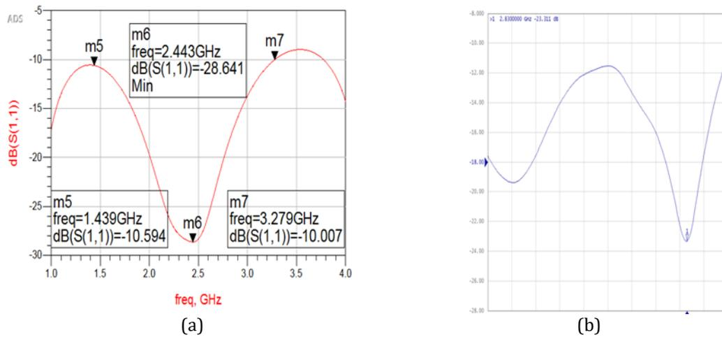
**Figure 7.** Simulated result of reflection coefficient ( $S_{11}$ ) of four-way power divider. (b) Simulated result of reflection coefficient ( $S_{11}$ ) of four-way power divider.
