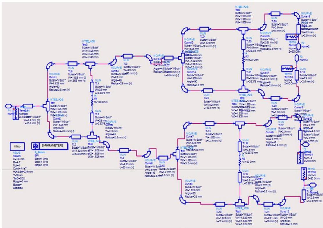
Figure 2. Four-way Microstrip Power Divider Design in Schematic Diagram.
