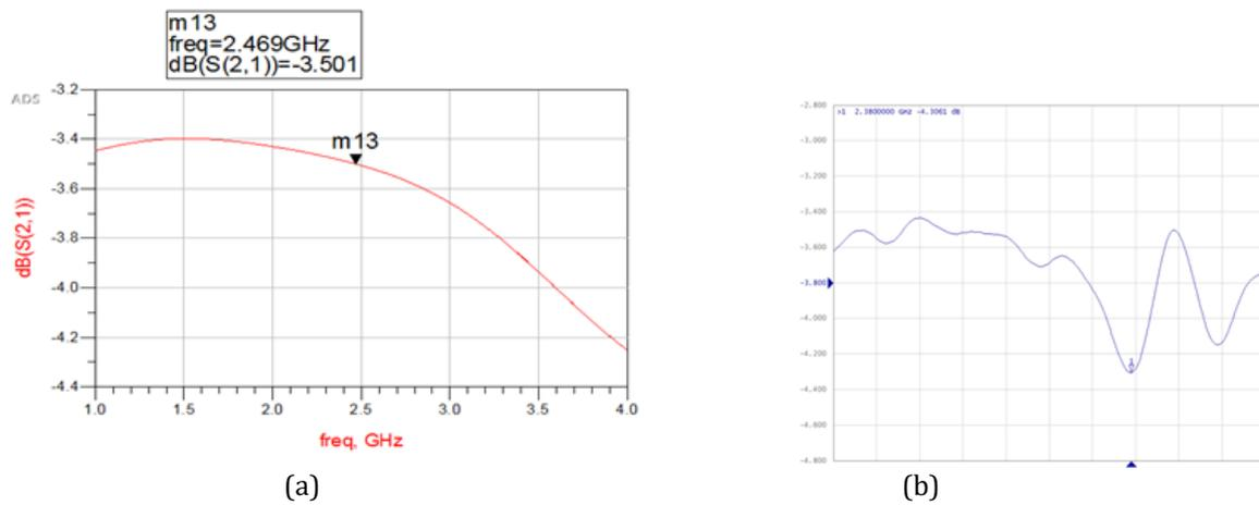
**Figure 5.** (a) Simulated result of insertion loss (S21) (b) Measured result of insertion loss (S21).
