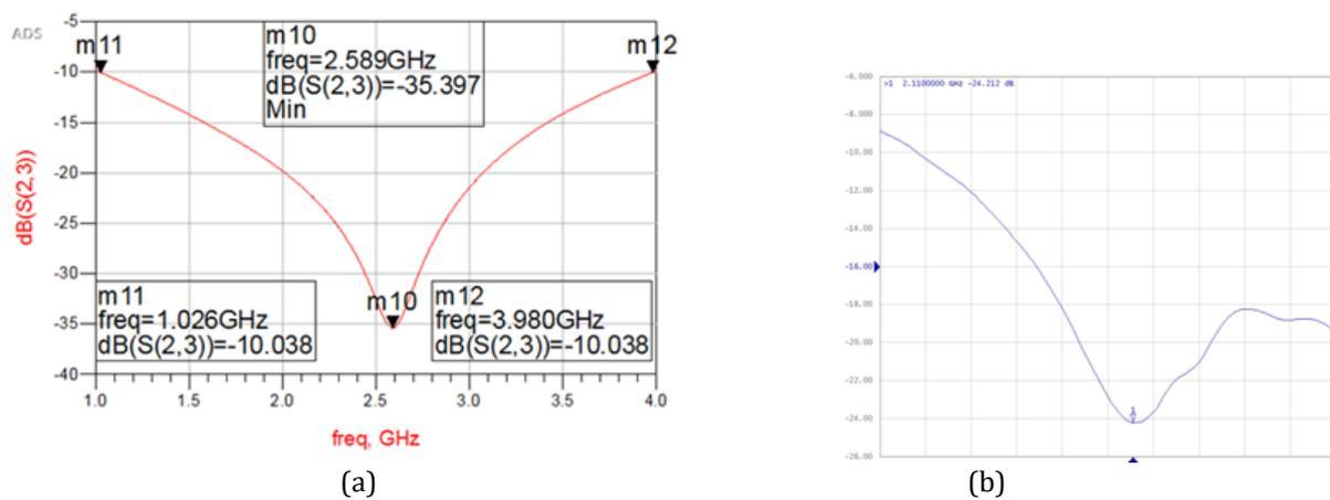
**Figure 6.** (a) Simulated result of isolation (S23) (b) Measured result of isolation (S23).
