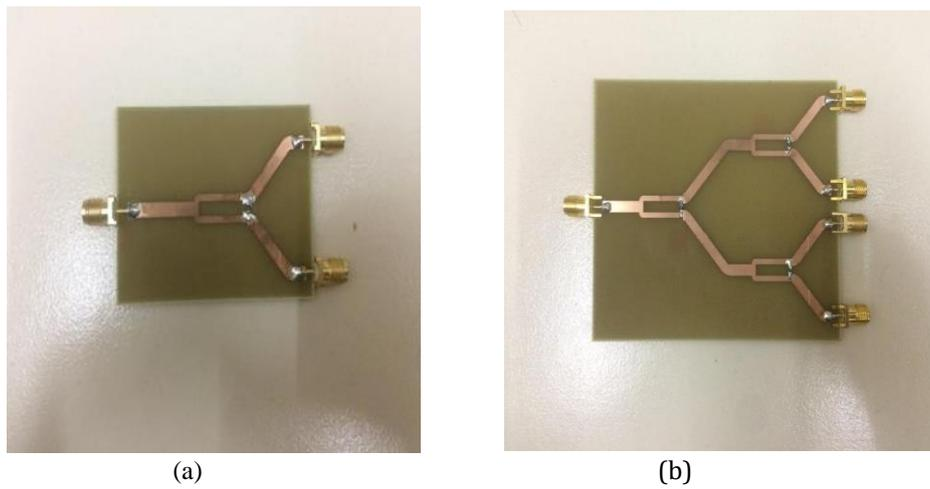
**Figure 3.** (a) Two-way Microstrip Power Divider (b) Four-way Microstrip Power Divider.
