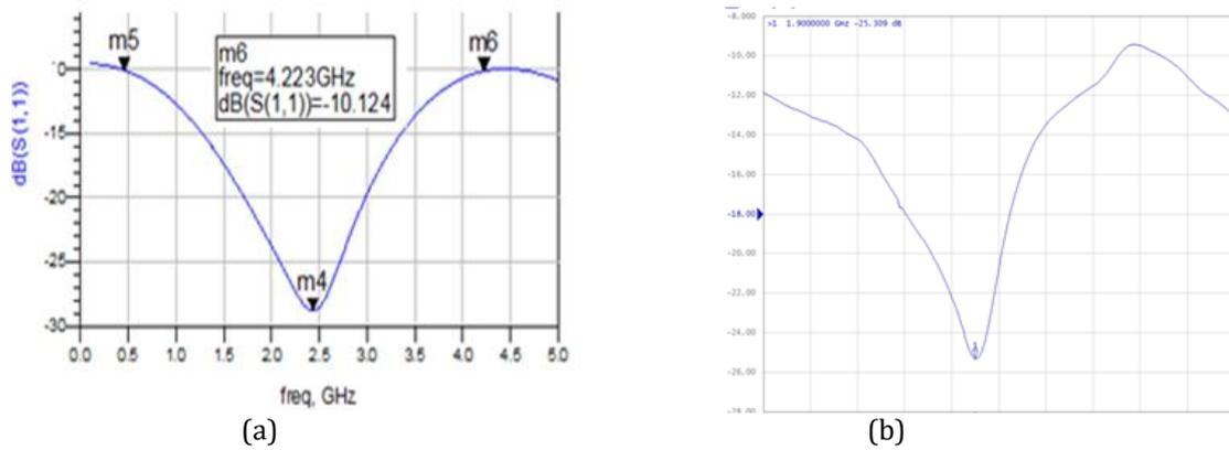
**Figure 4.** (a) Simulated result of reflection coefficient (S11) (b) Measured result of reflection coefficient (S11).
