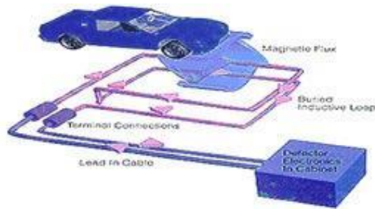
Figure 4. Inductive loop detector that is placed below the surface of the roadway
