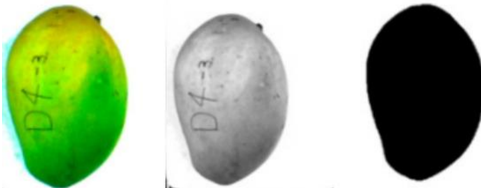
Figure 8. Processing Image from original RGB image, grayscale conversion and binary mask extraction for segmentation
