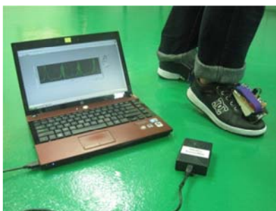
Figure 5: The Experimental Setup for Early Warning Fall Prevention System
